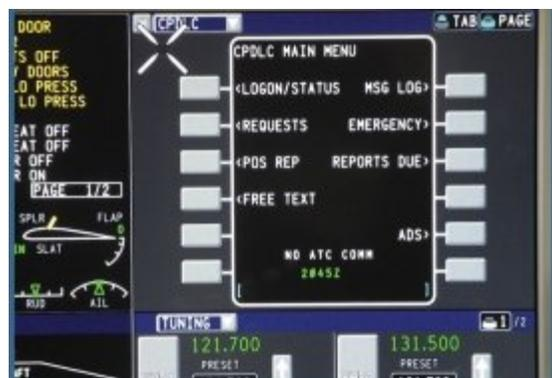
Controller pilot datalink communications (CPDLC), seen here in a Rockwell Collins Vision flight deck aboard a Bombardier Global Express, allows pilots and controllers to communicate effectively.
